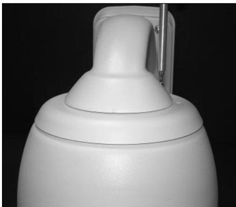
Photo 4N Tighten the Screws on the Pendant Arm
