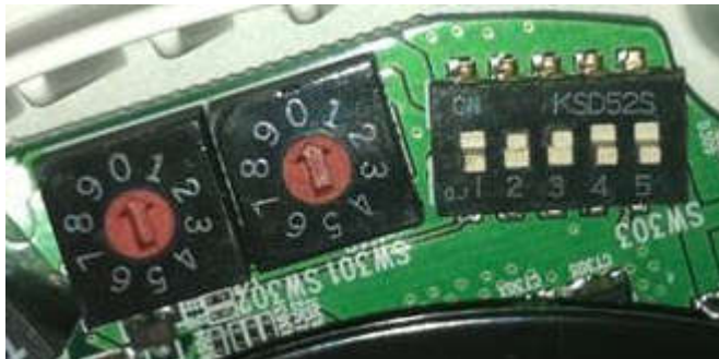
Figure 6.3: Close-up of Rotary Switches and Dip Switches
