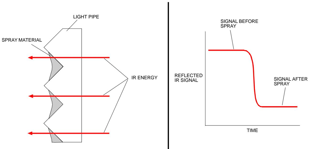
A dedicated IR photodiode senses the reduced reflected IR energy level, then sends a trouble signal to the security system indicating that someone masked the detector.
