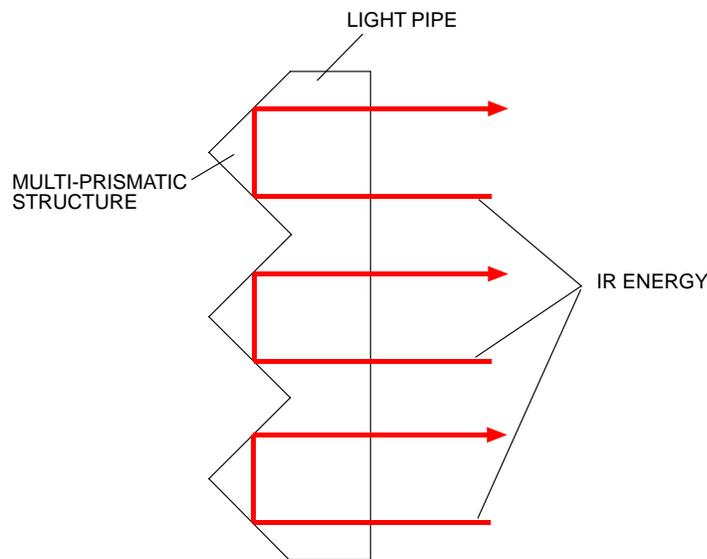
When the prismatic structure is coated with a spray material, the reflective properties of the prisms are negated, allowing the IR energy to pass through the prisms and out of the detector.
