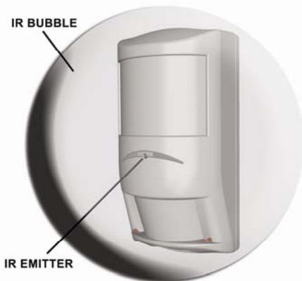
If the detector is blocked, an above-normal level of IR energy reflects back through the detector's lenses. The detector uses multiple IR photodiodes to detect the extra IR energy levels, then sends a trouble signal to the security system indicating that someone masked the detector.
