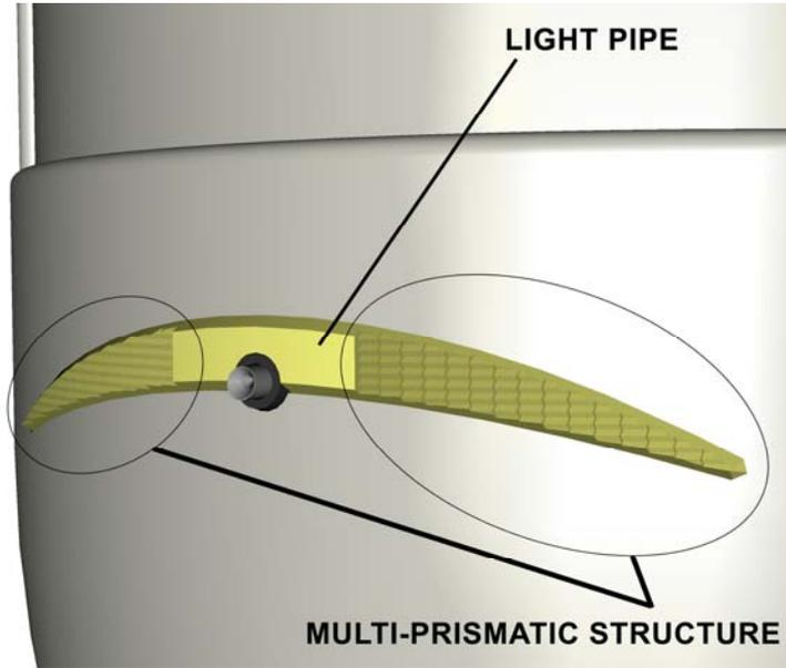
In normal conditions, the Retro Reflector structure reflects IR energy back into the detector. The IR energy does not pass through the prisms and out of the detector, and is reflected back into the detector where it is detected by a dedicated IR sensor.
