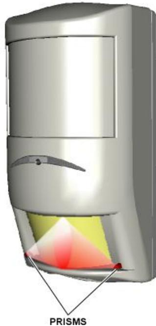
If the lens is masked, a photodiode receives reduced IR energy levels. The detector then sends a trouble signal to the security system indicating that someone masked the detector.
