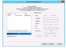
Select the device (checkbox) and press Add to use it and press finish
