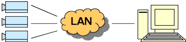
Fig. 4.1 Cameras connected over a local area network to a server PC running DiBos
