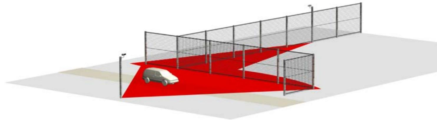
New Variable Field Illumination allows easy on-site adjustment of IR intensity and beam shape whether aimed along a fence (narrow beam) or directly at it (wide beam)
